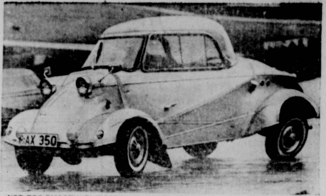
NOT TOO SMOOTH, BUT FAST —This bouncing baby car won't take any beauty prizes as it whips around a track at Brands, Hatch, England. It's a TG-500 Messerschmitt sports car, with a top speed of 90 m.p.h. and fuel consumption of 50 miles to the gallon. Has four wheels, too. (Other Messerschmitts have only three.)
