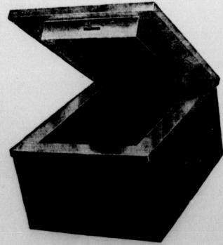
Made of heavy gauge steel inside and out, all electric welded, between these steel walls is 11/2 inches of solid Fire Proof Vermiculite Insulation which has over 300,000 tiny air cells to the square inch. It has the universally used toque and groove principle around the door with 1½-inch fireproof seal completely around it. Outside dimensions 14x111/2x 71/2 inches. Inside dimensions 81/2x11x 41/2 inches. Equipped with heavy standard type key lock, with two keys. Very attractive gray finish.
