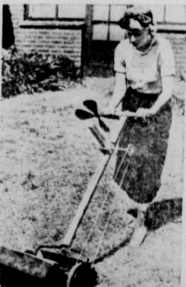
Hot weather hint: This resident of Kent, England, attached the blades of an old electric fan to the lawn mower. By means of a few gear wheels the fan revolves, blowing a cooling breeze as soon as the machine is pushed along the grass.
