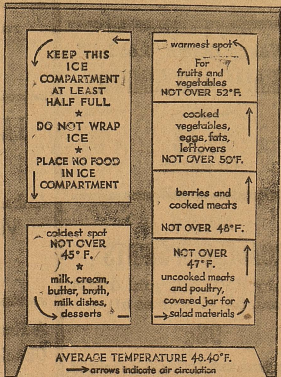
This diagram is from a chart entitled "Using the Temperatures in a Good Refrigerator," issued August 1, 1929, by the Bureau of Home Economics, United States Department of Agriculture. The refrigerator temperatures assume a room temperature of 75° F.
