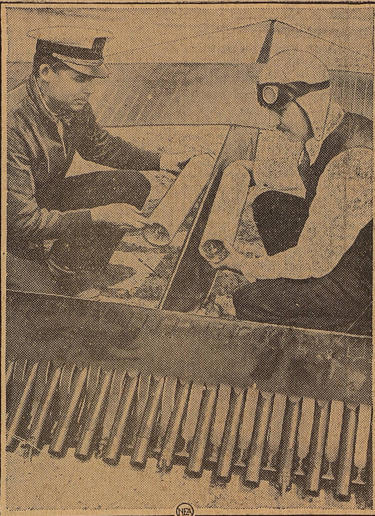
Maurice Poirier, left, an inventor of Burbank, Calif., is shown here with the model of a rocket plane which he hopes will attain a speed of 600 miles an hour. Both the model and the full-sized ship, which Poirier plans to build soon, will be powered by the fireworks spouting from the tubes in the tail, but the big plane will have a small gasoline motor for taking off and landing. The inventor and his assistant, Franklin Wallace, are shown here charging the model for an experimental flight.
