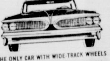
THE ONLY CAR WITH WIDE-TRACK WHEELS Dotted lines show conventional wheel positions. Pontiac's wheels are five inches farther apart. This widens the stance, not the car. Pontiac hugs tighter on curves and corners. Sway and lean are considerably reduced, ride is smoother, balanced, steadier.
