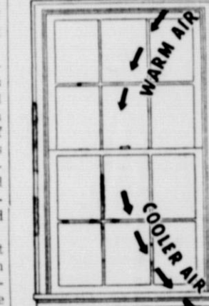
A single pane of glass cools warm air quickly. Cool air drops to floor causing drafts.
