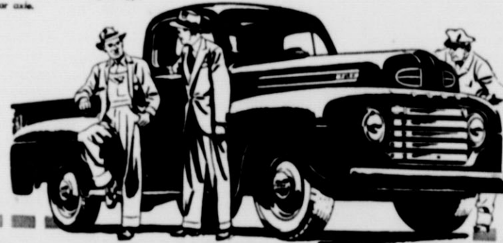
Ford 4 1/2 T. Half-Ton Pickup, G.V.W. 4,700 lbs. Choice of two engines, V-8 or Six. New integral type rear axle.
