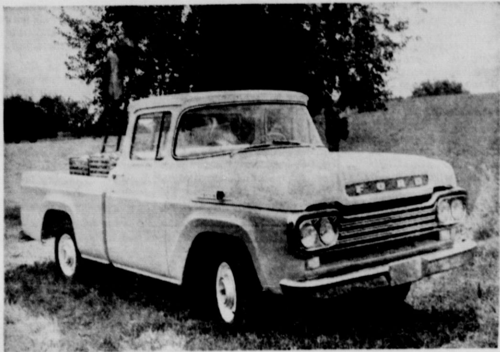
The popular F-100 pickup is one of 371 Ford truck models available in 1959. Dual headlights and a new Ford nameplate on the hood are standard features on the pickup models. With the 223 cubic inch six-cylinder engine — the most modern "six" in the industry — Ford offers greater economy in the high speed or increased load range. The pickup is available with either this Styleside body, which Ford pioneered with the 1957 models, or the Flareside body.
