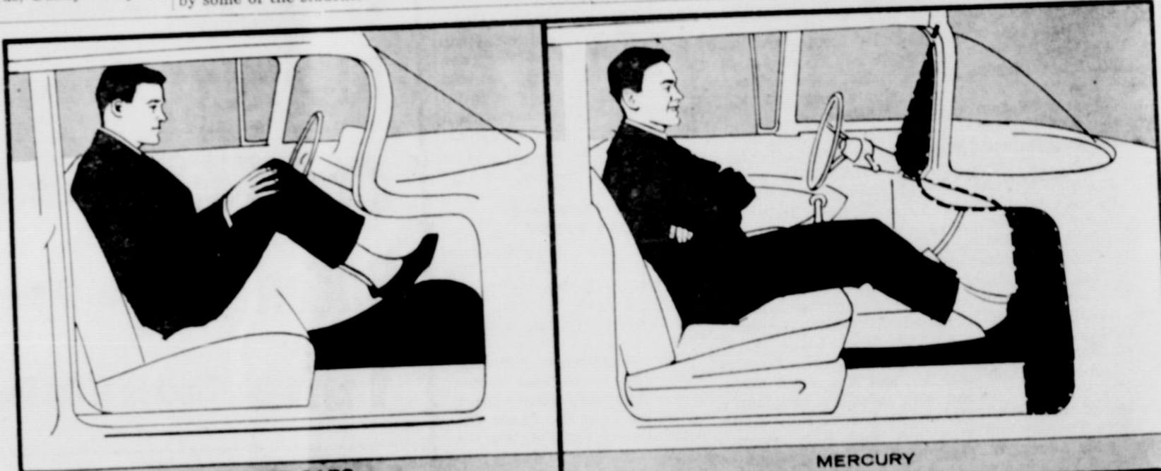
NARROW DOORS, CORNER POSTS STICK OUT. Other cars are actually issuing printed instructions on how to get in with dignity, without cracking elbows and knees. And note center hump now bigger than ever.
