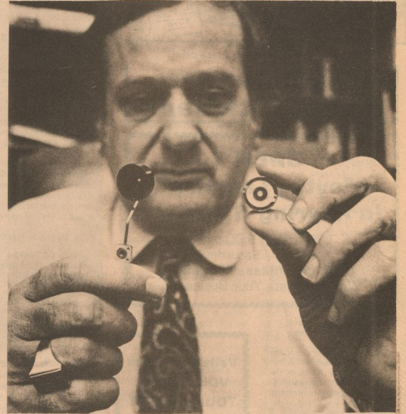
Baylor Otologist, Dr. Fred Owens, displays the external coil and holder for the cochlear implant system. When the external coil is placed on the skin directly over the implanted coil and activated with an electrical stimulator, the patient hears "environmental sounds."
