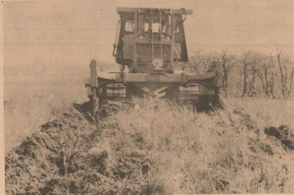
MECHANICAL BRUSH CONTROL accounted for over 5,000 acres of rangeland in the Upper Pease District being treated last year. Rootplowing and range seeding along with chaining were the principle methods used. Some chained areas have been set up for prescribed burns this spring to control resprouts and remove dead litter.
