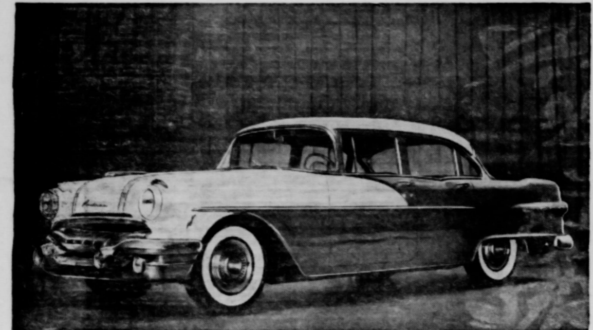
1956 PONTIAC 870 FOUR-DOOR SEDAN MORE POWERFUL — The popular Pontiac 870 four-door sedan offers more power and higher performance in 1956 with its bigger 205 h.p. Strato-Streak V-8 engine, and an improved Hydra-Matic transmission that gives smooth economical performance. Displacement of the 1956 Strato-Streak V-8 has been increased to 316.6 cubic inches and compression raised to 8.9:1. Exciting new colors in "Vogue" two-toning, sumptuous interiors and new styling features add new beauty to the four-door sedans, available in all three series.
