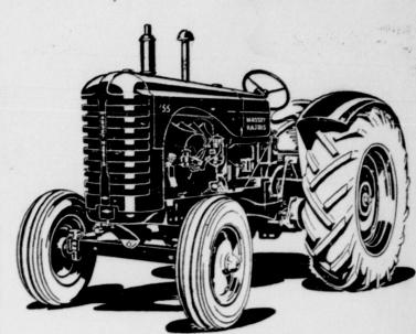
4-5 Plow Power 382 cubic-inch engine **Built-in** governor
