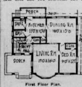
bathroom on the second. How these each one is shown on the plans. building itself is 36 feet wide and 32-feet deep. The entrance door from the porch leads into a small reception hall, out of which run the stairs to the second floor. To the right, con-nected with the reception hall by a double cased opening, is a living room, 14 feet wide and 16 feet deep. At the front on the corner is a bedroom, 9 by
