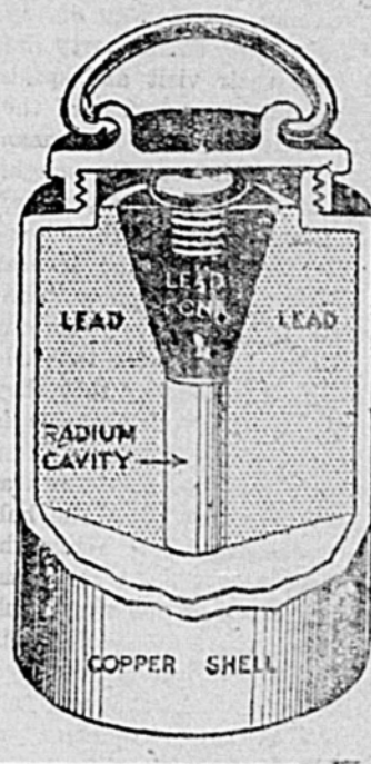
Construction of Container.
