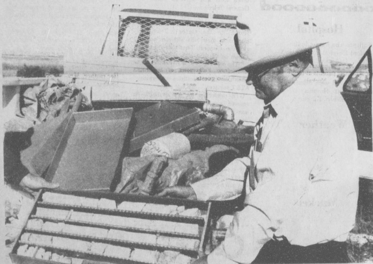
Judge Lee looks at core samples taken from the Palo Duro Dam site. Notice that the fourth sample from the top is very porous.
