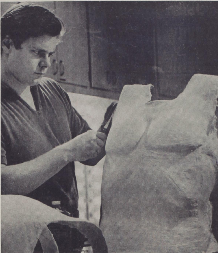
ARMOR FOR THE GODS — Biff Painter, Longview senior, demonstrates how a breastplate is molded in plaster, the first step in a process he devised for constructing lightweight armor from
