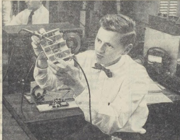
Winfield J. Giguere, here tuning the coils of an IF strip on an experimental FM receiver that uses the new high-frequency transistor.
