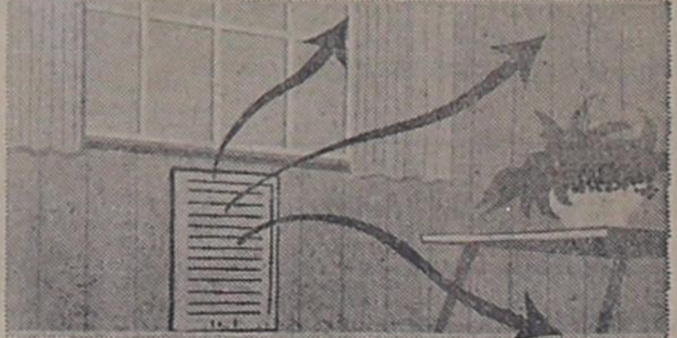
Electric wall panel heaters, with heating elements concealed behind a grille, provide radiant heat with natural or fan-forced convection. Also used as supplementary heat in baths or dressing rooms.
