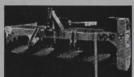
The Rock Rake attaches to a 3 point hitch. It will windrow rocks in the field just like hay. Then pick them up with the Rock Fork. The rock fork has quick attachments (depending on tractor type)! It can be used for rock picking, removal of brush, tree stomps, and large debris that needs to be removed and leave the soil behind.
