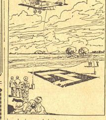
ing device used during the war and consisting of pieces of cloth spread on the ground and moved in shutter fashion, The message is attached to a line tied to the tops of two poles about six feet high The observer picks up the line by means of a hook dangled from the craft and the message is delivered as directed.
