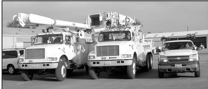
The trucks sent by Deaf Smith -- Bucket truck, Digger Derrick, and Service Pickup.
