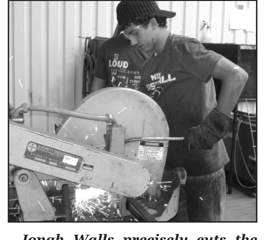
Jonah Walls precisely cuts the tubing to be used in the construction.
