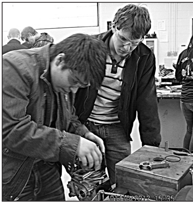
Diego Longley and Kyler Miller prepare to measure ring end gap of their piston rings.
