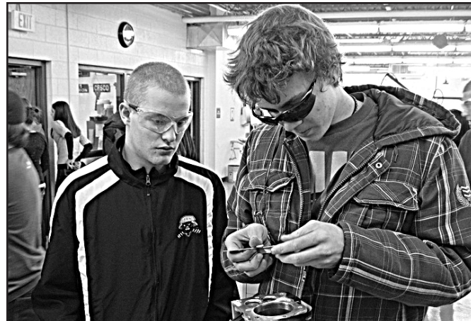
Mitchell Pinnell and Dakota Price use a feeler gauge to check tolerances.
