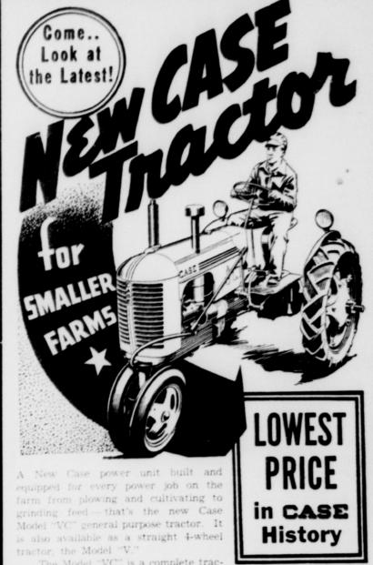
The Model "VC" is a complete tractor. It is not limited to plowing alone nor cultivating alone. It pulls a two-bottom plow, disk, drill or any other pull-behind implement and pulls them with a swinging drawbar which automatically locks into position when backing. Fitted with Easy on-Easy off clear-vision cultivator, the "VC" will quickly cover a wide range of
