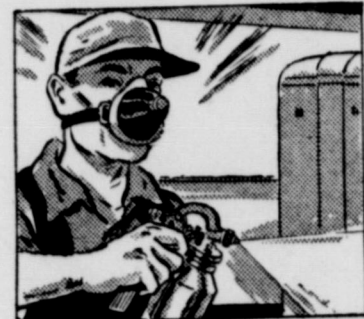
1. Not a gas mask, but a special nose mask to guard his breathing, is worn by this spray painter at his job in one of the General Electric plants.
