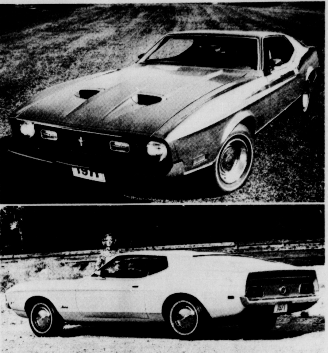
The 1971 Mustang Mach 1 (top) features a unique hood, grille and front bumper. The color-keyed, air-foil shaped, urethane molded bumper doubles as an efficient air-spoiler, improving high speed roadability. The Mustang Sports-Roof model (bottom) features a unique "flat roof" design in combination with Mustang's all-new sheet metal for '71.
