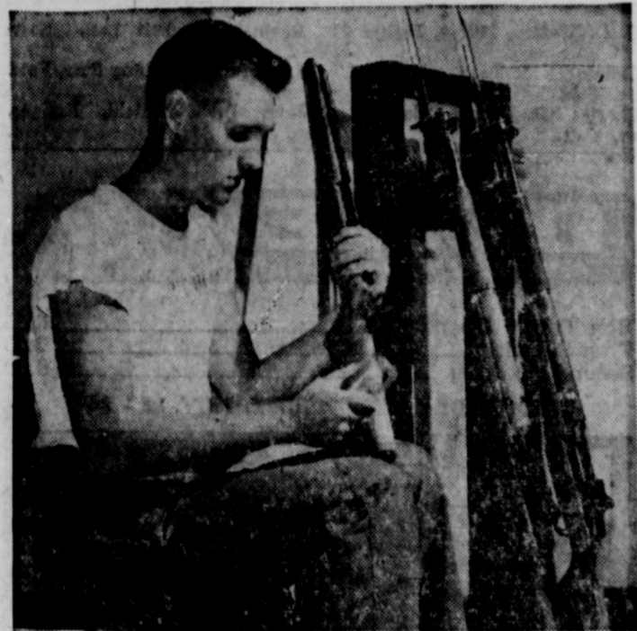
PRELUDE TO DUTY —Private Bernard R. Braun, Laurelton, L. I., one of the carefully selected soldiers from the Third Infantry Regiment, Fort Myer, Va., who stand guard at the Tomb of the Unknown Soldier, "bones" the stock of his rifle with a bottle. This smoothing process will be followed by many coats of lacquer. Rifles carried by sentinels are never handled with bare hands. Even finger rings are removed before each sentinel begins his guard tour.
