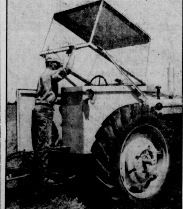
FARMER'S DREAM COME TRUE—Demonstrating the ultimate in farm luxury, a Doylestown, Pa., farmer lifts the glass and steel cover on an all-weather tractor. The cabin provides air-conditioning for the summer and heat for the winter. The tractor also has a push-button radio.
