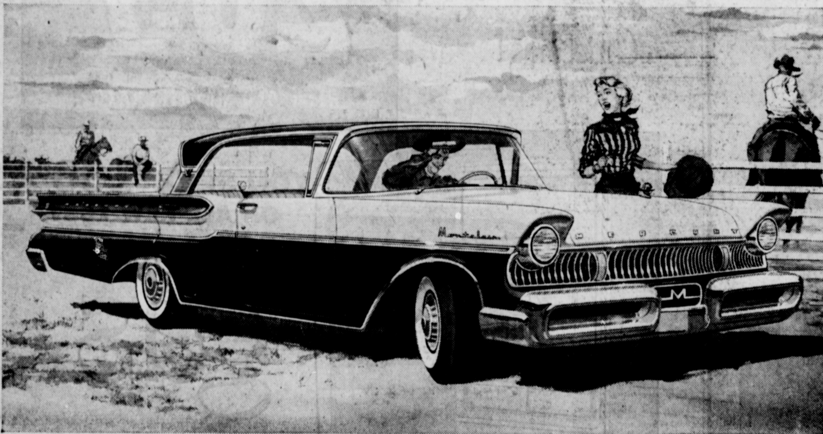
YOU ENJOY INCREASED HEADROOM—made possible by recessing the floor within the frame, and by the unique, straight-line design of the roof. Mercury's outside height is a sleek, shoulder-high 4 feet 8 inches.
