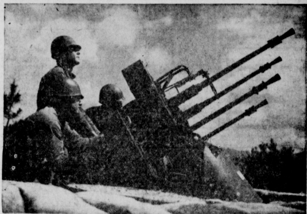
LEAD SPRAYER —When planes flew lower and slower during World War II, this anti-aircraft weapons system of four 50-caliber machine guns, towed or mounted on a tracked vehicle, proved to be a highly effective mobile defender of front line positions. With the advent of the jet age and combat in Korea, soldiers merely depressed the four barrels and found themselves with a tremendously lethal anti-personnel weapon, capable of firing 2400 rounds a minute, for cutting a swath through mass waves of attacking Communist troops.
