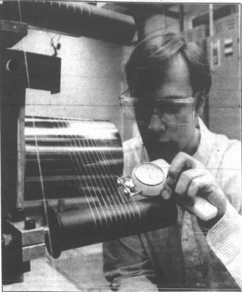
HIGH TENSION JOB —Senior research technician Marty Conroy uses a tensionmeter to monitor an experiment, testing the physical properties of nylon cord destined for truck tires, at Allied Corporation's research labs in Morris Township, N.J. Nylon filament is first strengthened with chemical additives and then pulled over godet wheels, shown here, to provide additional strength by tension-induced-molecular alignment and heat-curing. (AP Laserphoto)
