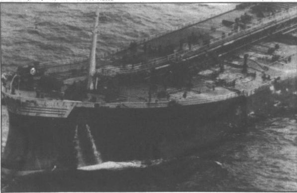
CRACKED TANKER-The 690-foot British tanker Alvenus rests on the bottom of a channel about 10 miles offshore from Galcasiu Pass, about 40 miles south of its destination of Lake
