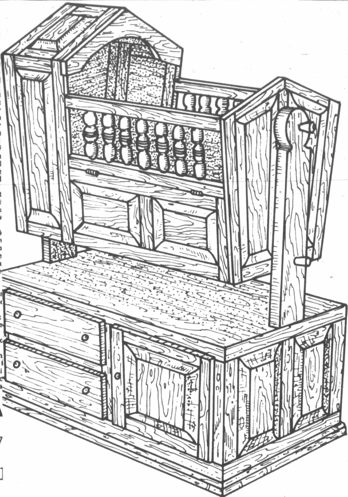
MAKE AN HEIRLOOM! — The cradle and chest combo in country style features raised-panel assemblies in sturdy frames. The cradle folds down sides and a protective hood. The chest features two drawers and a decorative front panel.
