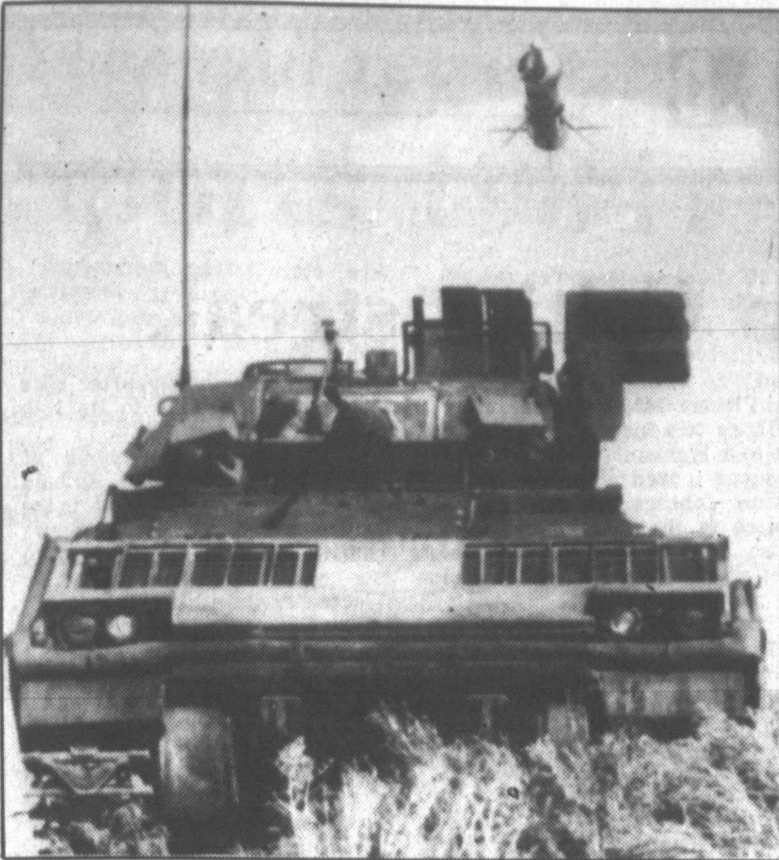
BEEFED-UP MISSILE TESTED — A TOW 2 anti-tank missile, an improved version which features a better guidance system and a more potent warhead designed to defeat advanced enemy armor, flies from the launch tube of the U.S. Army's Bradley Fighting Vehicle during recent tests.
