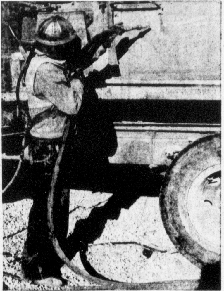
CLEANING A TRUCK — One of A. L. "Red" Weatherred's co-workers is shown cleaning — sand blasting — one of the Transmix Concrete and Material Co. concrete mixing trucks. This job is an illustration of the variety of work Weatherred does by sand blasting; gasoline refineries, gas plants, tanks, (interior and exterior), brick, stone and metal structures and buildings. Red's work is efficient, fast, neat. Call him at 4-4001 or 4-6881.
