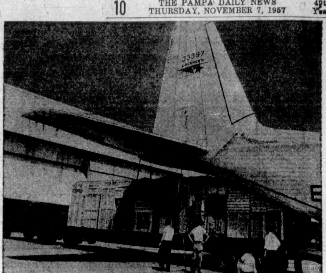
ALL DELIVERIES IN REAR—A massive cargo of 22 tons is loaded in a matter of minutes into Lockheed's new commercial air freighter, the Hercules. The 320-mile-an-hour plane, shown here in a demonstration at Marietta, Ga., is America's first turbo-prop cargo carrier which permits straight-in, truck-and-dock-level loading. Tests, using conveyor belts to speed handling of cargo, have proved that the huge 4,300-cubic-foot maw of the craft can be filled in a few minutes' time, compared to several hours required for other transports.
