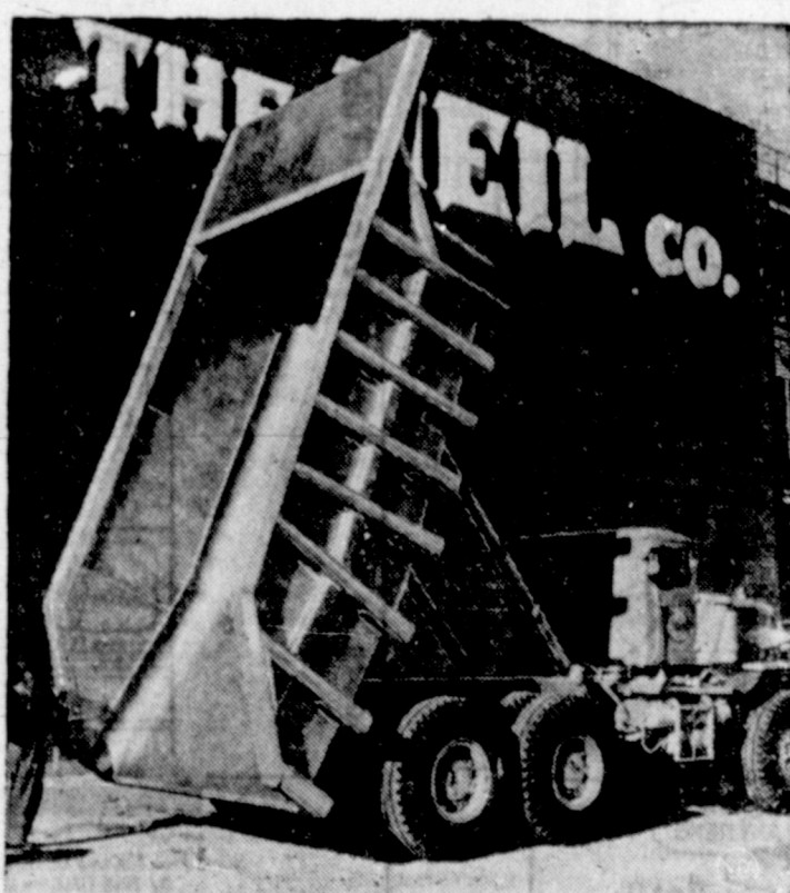
BIG AS A TRUCK —This huge aluminum body with a capacity of 37 1/2 cubic yards is the largest ever built for a dump truck. The truck is 30 feet, 3 inches long, 12 feet, 4 inches wide, 11 feet, 11 inches high and weighs 54,000 pounds. Built by Mack Trucks for the Aluminum Company of America, it will be used in bauxite mining operations in the Dominican Republic. The truck, for off-highway use, is powered by a 335-horsepower turbocharged diesel engine, carrying a load of 67,000 pounds.
