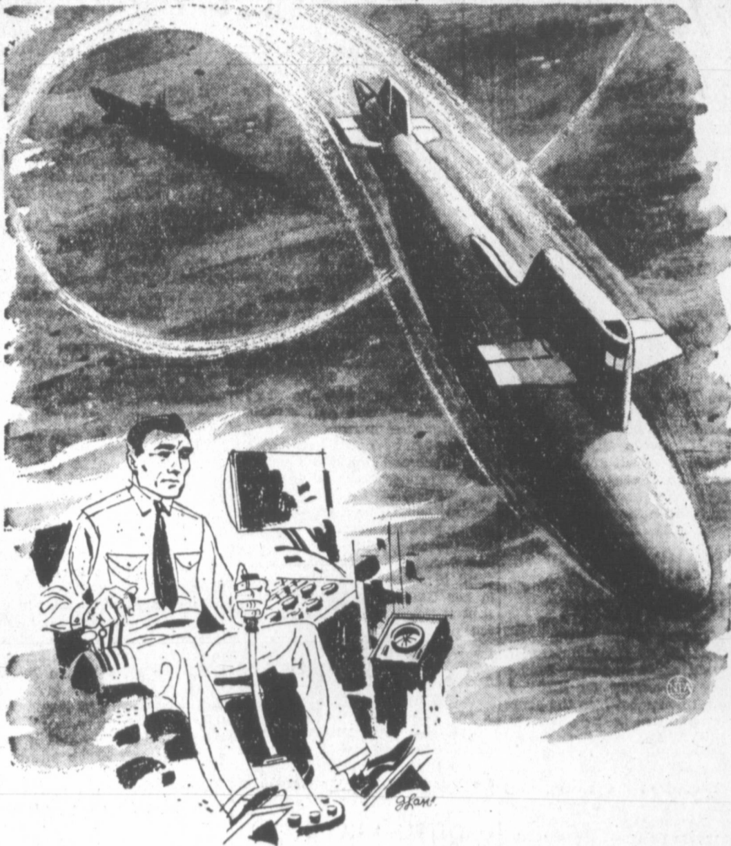
"AQUABATIC" SUB — The Skipjack, the Navy's newest nuclear submarine, promises to introduce new tactics into the art of undersea fighting. The 250-foot Skipjack, shaped like a shark, will be the fastest undersea craft ever built. An experimental sub, the Albacore, is the hull prototype for the Skipjack. The Albacore holds every sub speed and maneuverability record in the world. Sketched above by NEA artist John Lane, the Skipjack is shown making an aircraft-type pass at an "enemy" sub. The sub's driver (inset) will be called a "pilot." He will use a "joy stick" for controls, and be able to direct his sub in "aquabatic" maneuvers like a fighter pilot. Performance figures on the Skipjack are secret, but it is believed capable of doing 35 miles per hour submerged. Pitted against the conventional Russian sub of today the Skipjack would be like a jet fighter attacking a slow-moving cargo plane.
