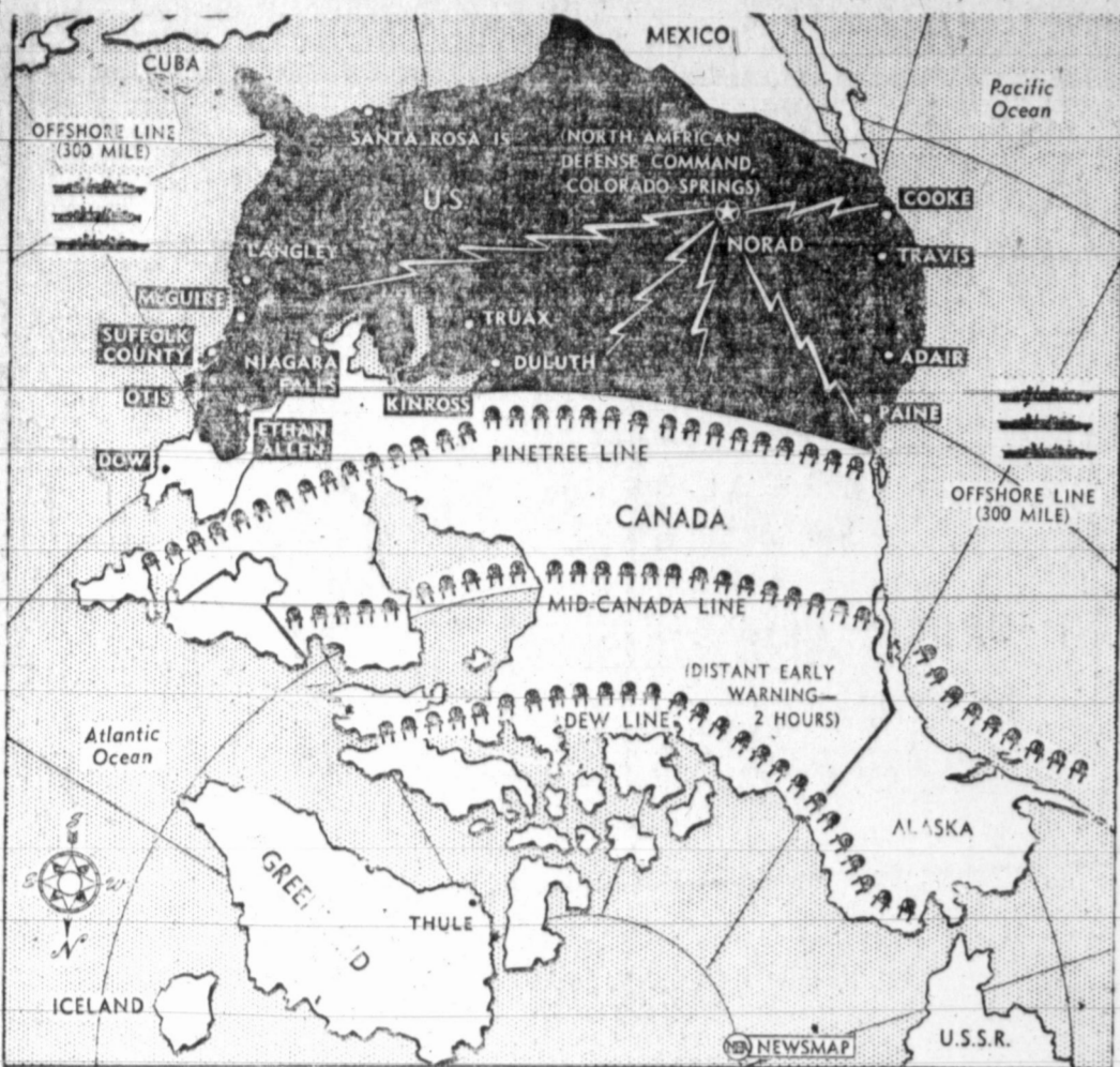
NEW MUSCLES FOR NORAD —Looking south from the North Pole gives this enemy bomber's view of some of this continent's defenses against attack. Behind the radar picket fences of DEW, Mid-Canada and Pinetree lies the brain center of NORAD, the North American Defense Command. Advanced air bases in Iceland, Greenland and Alaska, and offshore radar-equipped ships, blimps and planes are also part of the defense system. Soon to be added to this picture will be a ring of launching sites with a potential range of 200 to 400 miles outside our borders. These are the 15 Bismarck guided missile bases (white type on Newsmap) which NORAD has announced will be built. Some are already under construction; other sites are planned for the future.
