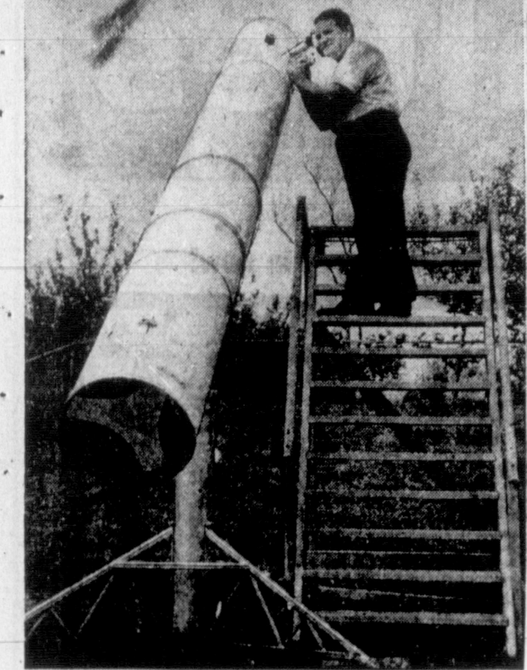
FRONT ROW SEAT—Though he can't take a trip to the moon in person, Charlie Norris of Cincinnati, Ohio, has the next best thing—a 1,800-power homemade telescope which brings the moon to within an apparent distance of 130 miles from his back yard. Charlie, operator of a TV service, got the bumper after the first Sputniks were launched and built the 13-foot reflector for $300 and a year of part-time work. It took him seven months to grind the 12 1/2-inch mirror alone. The result is the most powerful scope in the area, so that has
