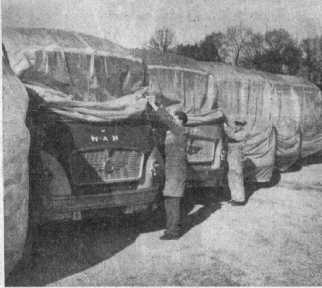
IN THE BAG —New buses come in plastic bags at a vehicle factory in Munich, West Germany. Lined up for shipment, each bus is covered with a bag weighing about 30 pounds and costing $170. They're used as protection, and keep the vehicles bright and shiny on the rail or truck journey to their eventual buyers.
