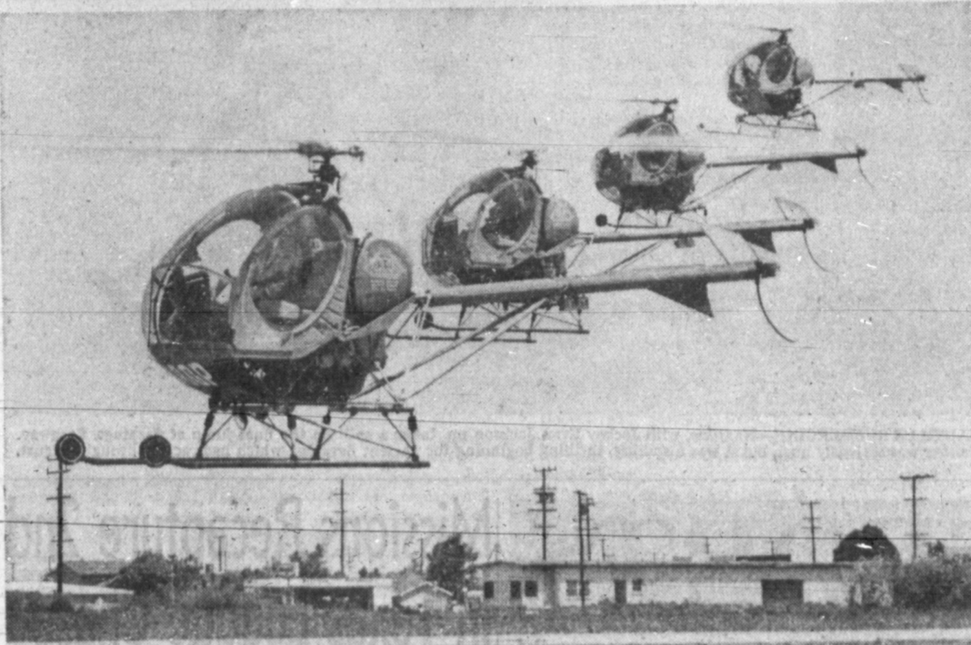
WHAT DAT? —Looks like a doodlebug invasion from outer space, but it's actually four Hughes Model 269A helicopters landing tandem style at the Hughes Tool Company in Culver City, Calif. Scheduled to go into immediate commercial production, the new whirlybirds cruise at 85 miles an hour, have a ceiling of 11,000 feet and a range of 195 miles. They have a gross weight of 1550 pounds and can carry 635 pounds.
