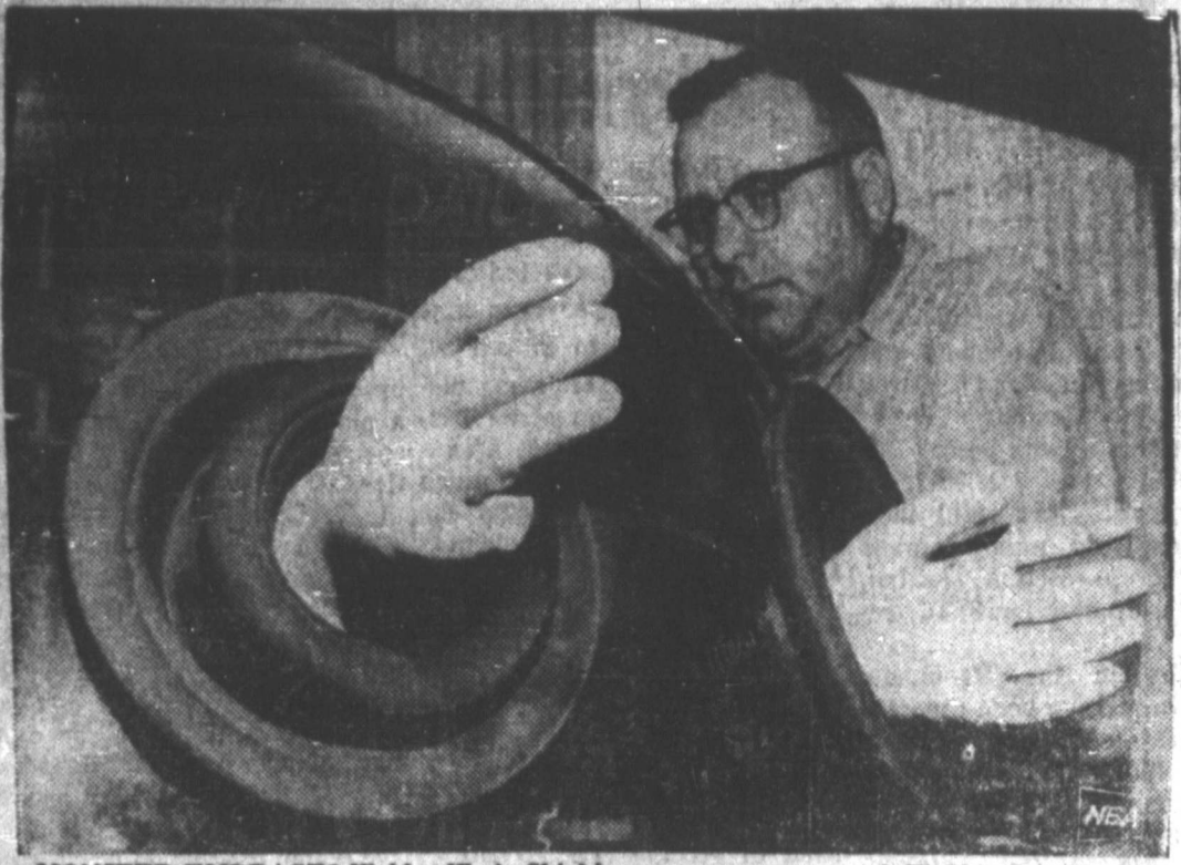
MONSTER EMBRACE? Welder W. A. Shields appears unconcerned. The hands actually are gloves forced inside out by gases used to purge a welding chamber. The chamber was purged to create an inert atmosphere for working on certain metals. Shields puts his hands in the gloves to work inside the bubble.
