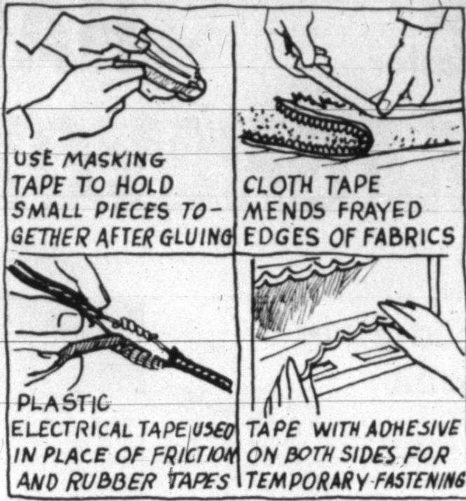
USE MASKING TAPE TO HOLD SMALL PIECES TOGETHER AFTER GLUING. CLOTH TAPE MENDS FRAYED EDGES OF FABRICS. PLASTIC ELECTRICAL TAPE USED IN PLACE OF FRICTION AND RUBBER TAPES. TAPE WITH ADHESIVE ON BOTH SIDES FOR TEMPORARY FASTENING.
