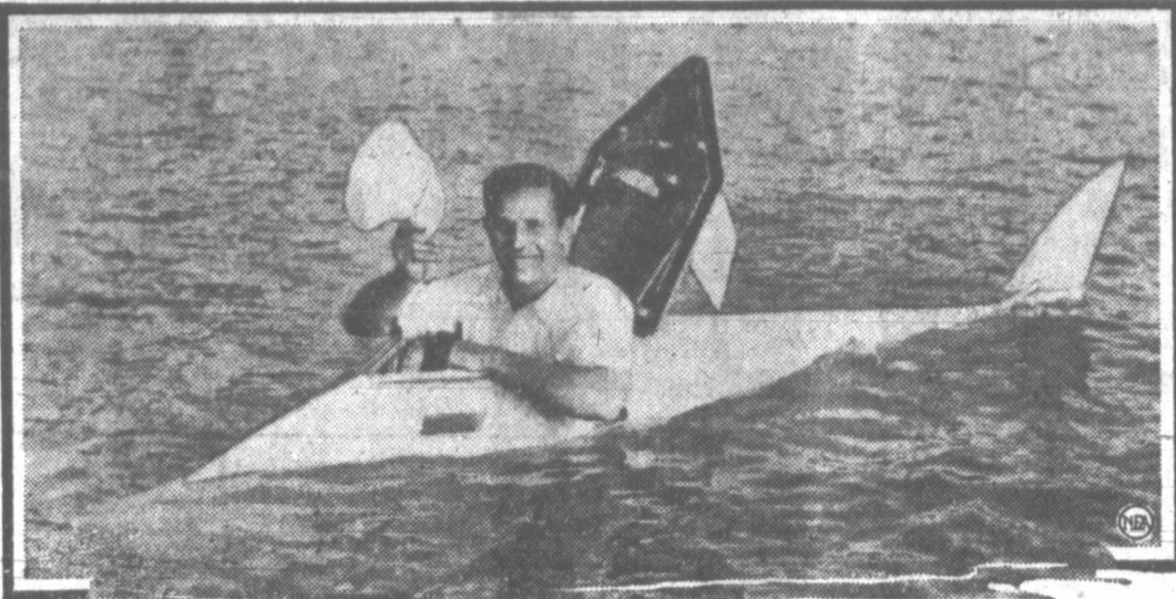
It looks like a big metal fish, but it's really a submarine, vest pocket type. Ten feet long and weighing 1000 pounds, it has a speed of six miles an hour and submerges to a depth of 17 feet. The inventor, Barney Connett, 30, of Chicago, is shown as he demonstrated the craft at the Jackson Park Yacht Club in Chicago.
