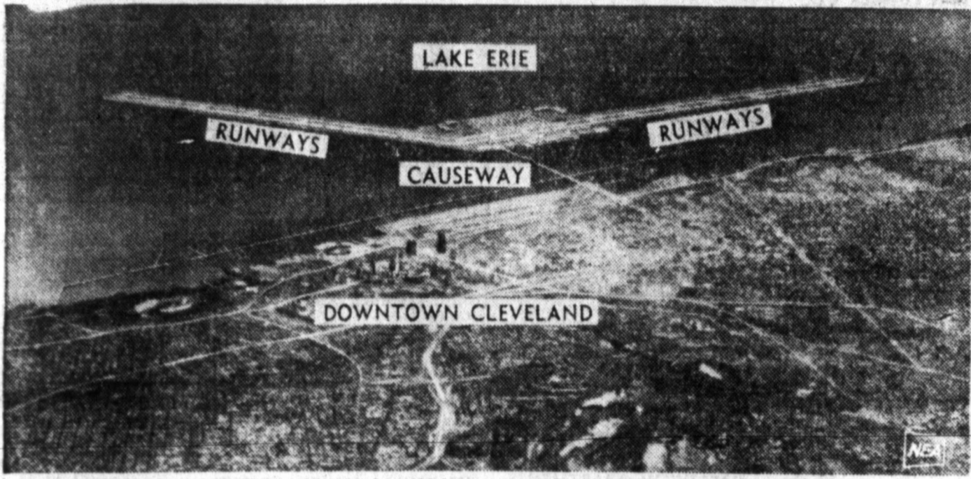
PROPOSED SUPER AIRPORT at Cleveland would be constructed on landfill 20 feet above the surface of Lake Erie and connected with the center of the city by a mile-long causeway. Runways would be two miles long. All approach and takeoff patterns would be over water, eliminating noise from flights over populated areas.
