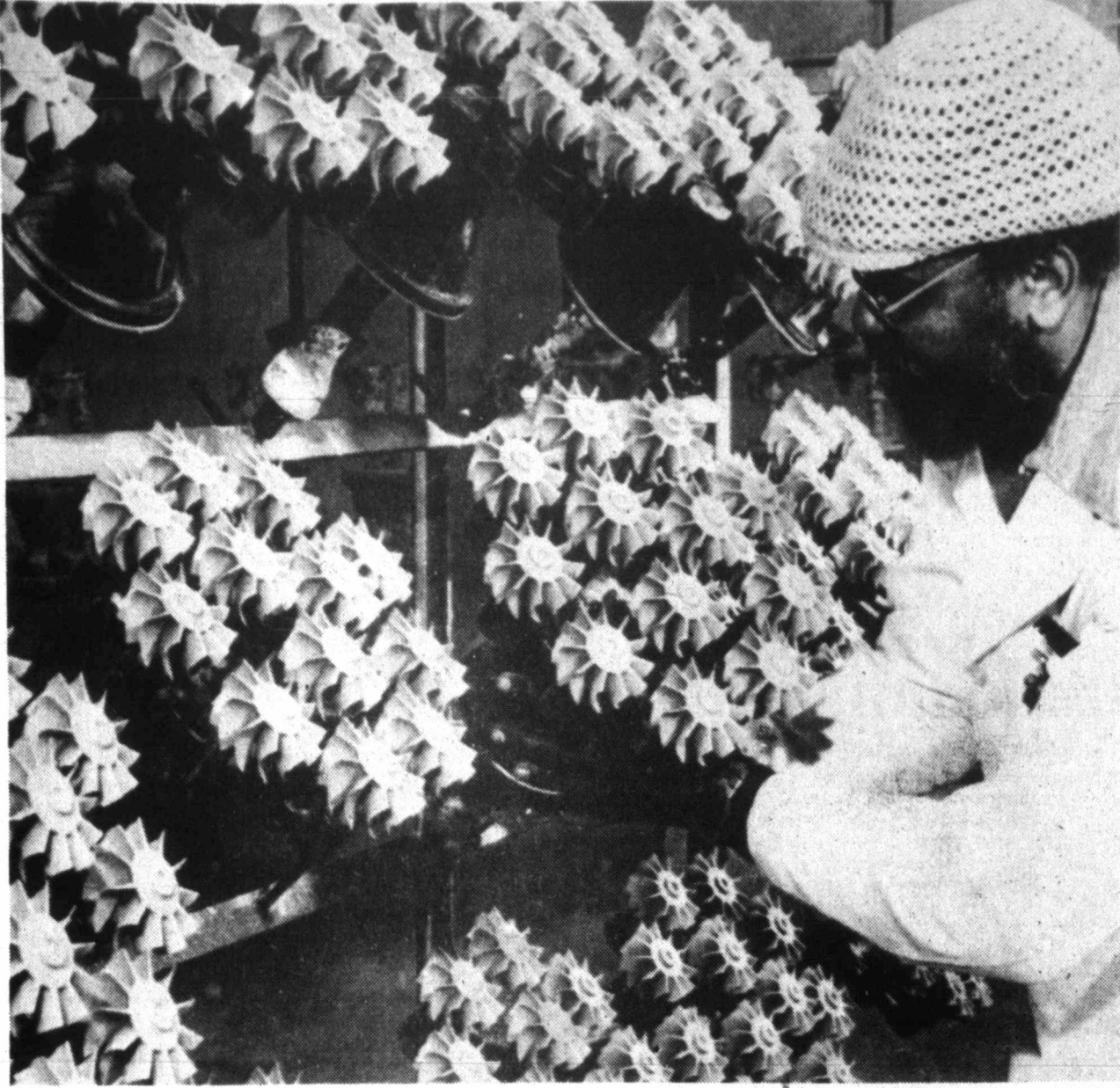
TURBINE BOUQUETS. A mold handler at the Garrett Corp. in Torrance, Calif., removes wax turbine molds from racks at the company's casting facility. Each wax wheel is a pattern for a steel casting, a component used in turbochargers for boosting engine power on tractors, trucks, off-highway vehicles and automobiles. (AP Laserphoto)
