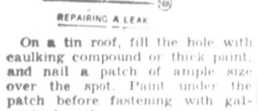
REPAIRING A LEAK On a tin roof, fill the hole with caulking compound or thick paint, and nail a patch of ample size over the spot. Paint under the patch before fastening with galvanized nails.
